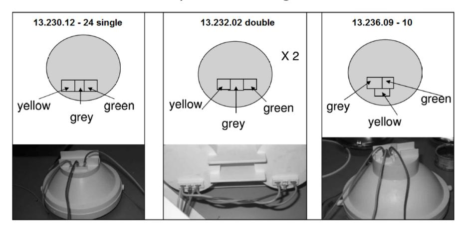
Each cable has its position and you must respect cable colour in each location yellow: common grey: deep light green: short light
