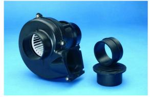
5000 hr. motor life for the harviest of application CAPACITY: 260 mc. per hour DIMENSIONS: 195 x 173 x 190 mm PORT CONNECTIONS: Inlet: 75 mm - Outlet: 72 mm CD. 5500001212 12 V. Amp draw 4.5 A. CD. 5500001224 24 V. Amp draw 3.5 A. Casing is entirely moulded in strong nylon plastic, with motor completely enclosed in a plastic compartment for added safety and protection. Screws and shaft in stainless steel. Homologated by the Italian Navy Register (R.I.N.A.).
