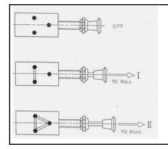
\*\*\* 20410/11 When pushed in all the way, the switch is turned off. When pulled to the first stop, the first circuit is activated. At the second stop both the first circuit and the second circuit are activated.
