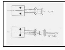
\* 20390/1 When pushed, the switch is turned off. When pulled, the circuit is activated.
