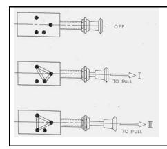
\*\* 20400/1 When pushed in all the way, the switch is turned off. When pulled to the first stop, the first circuit is activated. At the second stop the first circuit is deactivated and the second circuit is activated.
