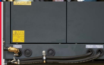
Input/Output fuel pipe
